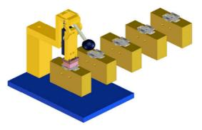
When testing a new specific component size, you need to select the correct corresponding Midsection Assembly. This insures that the component will make contact at the correct areas on the microstrip line and the ground pad. If this is not accomplished, you will have annomalies in your data due to incorrect spacing between the ground and RF signals on the device.
