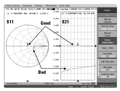
Figure 10. Confirmation of device contact condition
