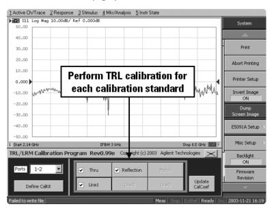
Figure 5. Performing TRL calibration
