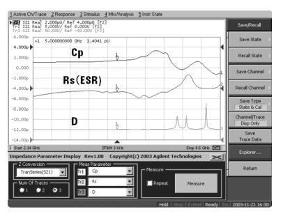
Figure 12. Measurement results of SMD capacitor using impedance parameter display software
