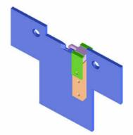
A midsection is inserted into the test fixture. The size of the midsection determines the size of the DUT to be tested. The midsection assembly has two guide holes for alignment with the test fixture. The chamfered side of the alignment holes is on the input side of the test fixture on all midsections.
