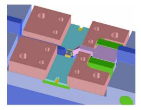
DUT guides shown in place with the DUT and the midsection. The DUT guides are removed during calibration.
