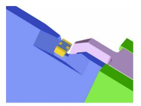
The midsection has a fixed and a movable ground contact. The movable ground contact slides down a 45 degree ramp. As it slides down, it moves toward the DUT and makes ground contact. The brass push pin of the pusher assembly pushes the movable ground contact onto the midsection. The movable ground contact is automatically retracted when the brass push pin moves up.
