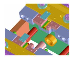
Two DUT guides help place the DUT evenly onto the RF contacts (DUT guides are shown in blue).
