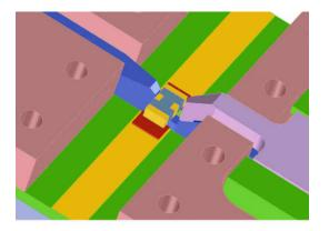
For testing, the DUT is placed onto two microstrip launches with DURA contacts.
