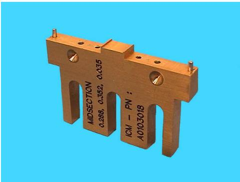
The MMIC Midsection Adapter dimensions have to match the MMIC Carrier Assembly in order to hold and position the DUT properly in the test fixture.
