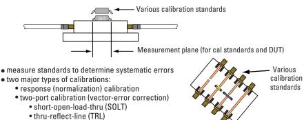
Direct measurements have the advantage that the precise characteristics of the fixture do not need to be known beforehand. They are measured during the calibration process. The simplest form of direct measurement is a response calibration, which is a form of normalization. A reference trace is placed in memory and subsequent traces are displayed as data divided by memory. A response calibration only requires one standard each for transmission (a thru) and reflection (a short or open).
