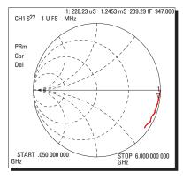
watch out for "negative" capacitance (due to long or inductive short) adjust with negative offset-delay in open <or> positive offset-delay in short
