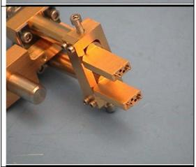
An Adjustment screw on each side can be used to set the distance between the RF-pins. The spring loaded Ground pins can be positioned using different ground pin location holes.
