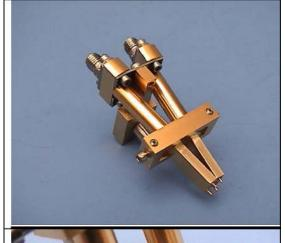
The Adjustment screws can be locked in place by two setscrews.
