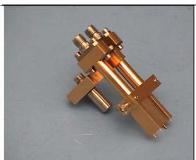
The ICM Differential TDR Probe can be adjusted over the range 0.100" – 0.500"
