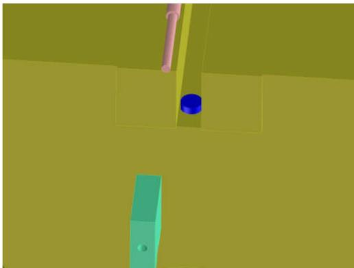
Keep the Transition upright, and prevent the small pin from falling out. This pin pushes up the dielectric sleeve and spring-loads the RF pin. The pin in the picture is shown in blue.
